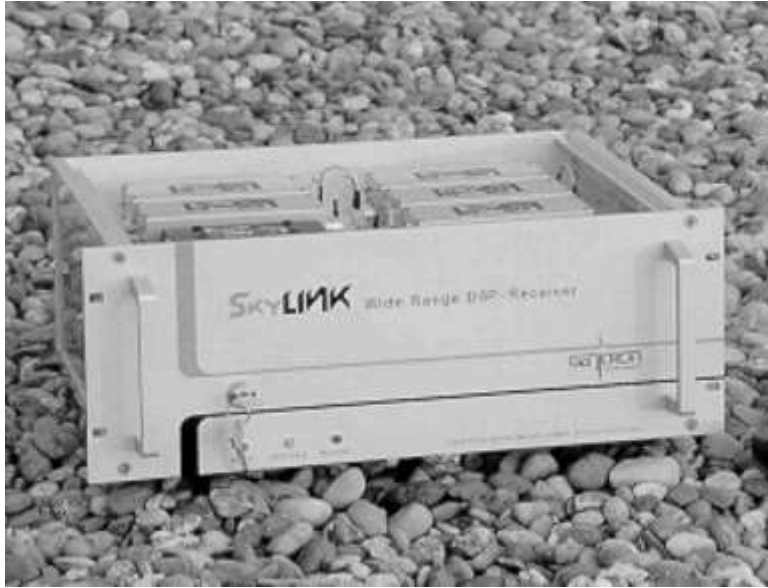
FIG. 7: The indoor-unit, a heavy 19" plug-in, containing three different system layers:
