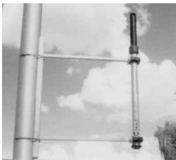
FIG. 4: Self-contained gamma monitor (incl. radio module) fixed to a light pole. The tubular-shaped metallic construction guarantees hermetic seal over many years. The lambda/4 antenna rod is emitting through the black POM-cap on the top.
